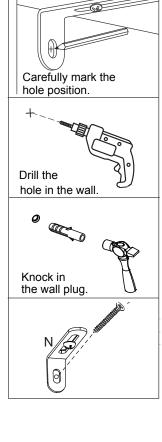
When you are satisfied with the position and the wall fixing method chosen holds each bracket firmly in position, tighten screws (N).
