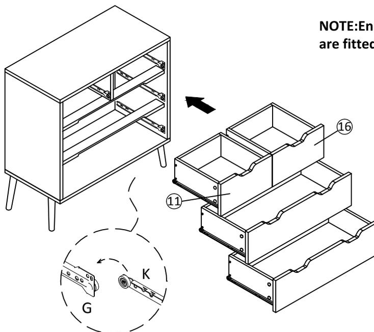
NOTE: Ensure left and right hand drawers are fitted into the correct drawer slots.
