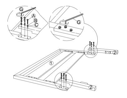
STEP 3 Required Fitting: D x 28 pcs 5 x 14 pcs 6 x 2 pcs 7 x 4 pcs Fitting Support Leg with Slat and Slat Support. Attach Slat to Side Rail.
