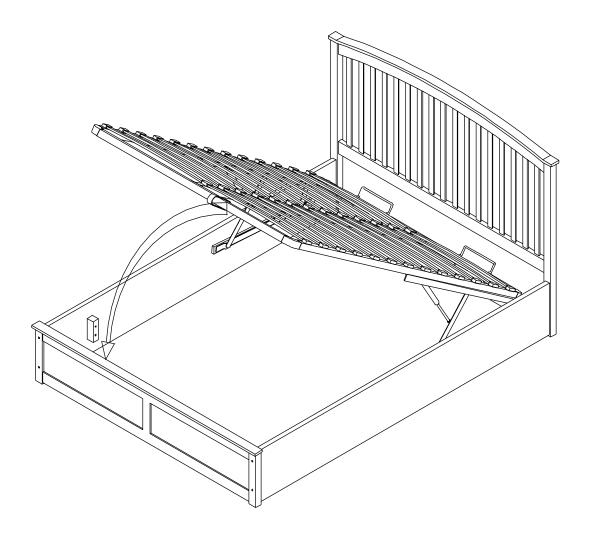
Lift with the strap (H13) and close with the strap. The strap should always be accessible. Take care not to lean over the bed when lifting, if the mattress is thin and light, the frame may rise quickly. The speed of closing will also depend on the weight of the mattress so always keep fingers well clear of the metal frame.
