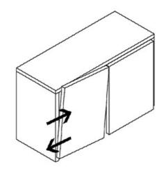
**Lateral Adjustment** by adjusting screw
