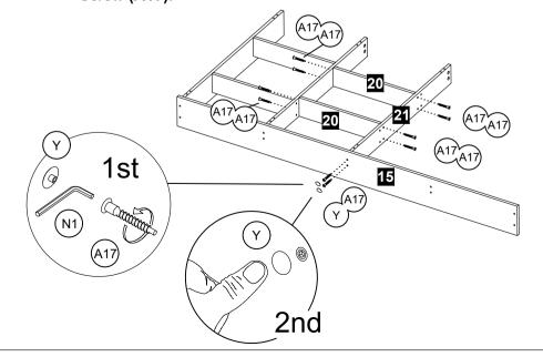
Then, assemble panel no. **20** & **21** together using 6.3 x 40mm Crosshead Screw **(A17)**.
