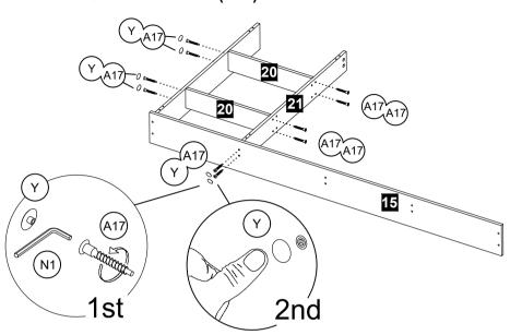
Assemble panel no. **20** & **21** together using 6.3 x 40mm Crosshead Screw **(A17)**.
