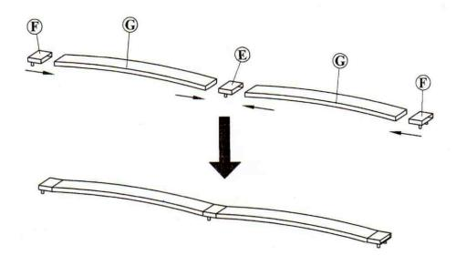
Step 4 : Align the pins on the Plastic Slat Holders (E) (F) to the holes along the Centre Rail (D) and the Siderails (C). Gently tap them into the holes. Tap the corners of the Plastic Slat Holders (E) (F) to knock them into place with rubber mallet. ( NOT provided )
