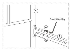
$\underline{\textbf{IMPORTANT:}} \ \ \text{Do not tightly secure the screws before completing Step 2}.$
