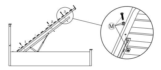
Step 10: Adjust the bed base making sure that the distance to the footboard is approximately 15 mm to above. Tighten all bolts and screws now.
