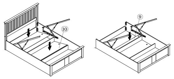
Step 9: Attach the bed base to the hydraulic frames using hardware part M. Fix the bolts starting from area 1 and finishing in area 3 – do not fully tighten the bolts yet.
