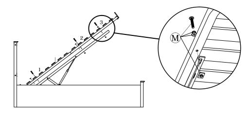
Step 10: Adjust the bed base making sure that the distance to the footboard is approximately 15 mm to above. Tighten all bolts and screws now.
