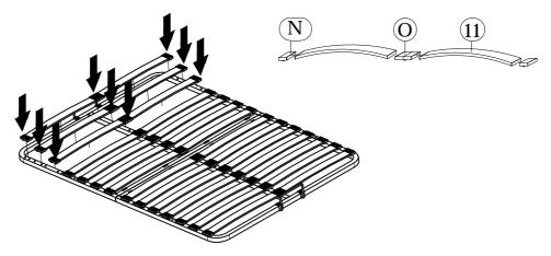
Step 8: Insert the small base panel (9) and large base panels (10).
