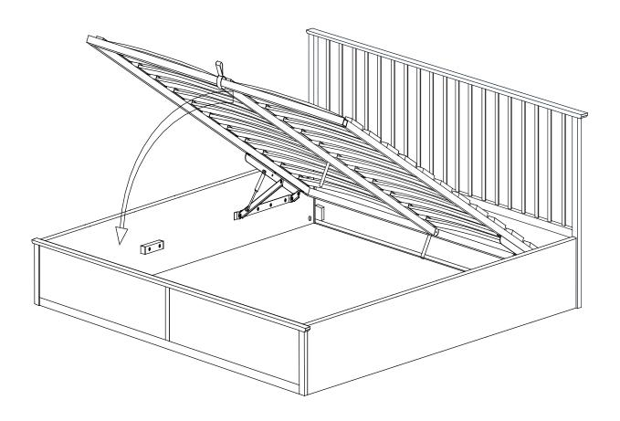
Lift with the strap (H13) and close with the strap. The strap should always be accessible. Take care not to lean over the bed when lifting, if the mattress is thin and light, the frame may rise quickly. The speed of closing will also depend on the weight of the mattress so always keep fingers well clear of the metal frame.
