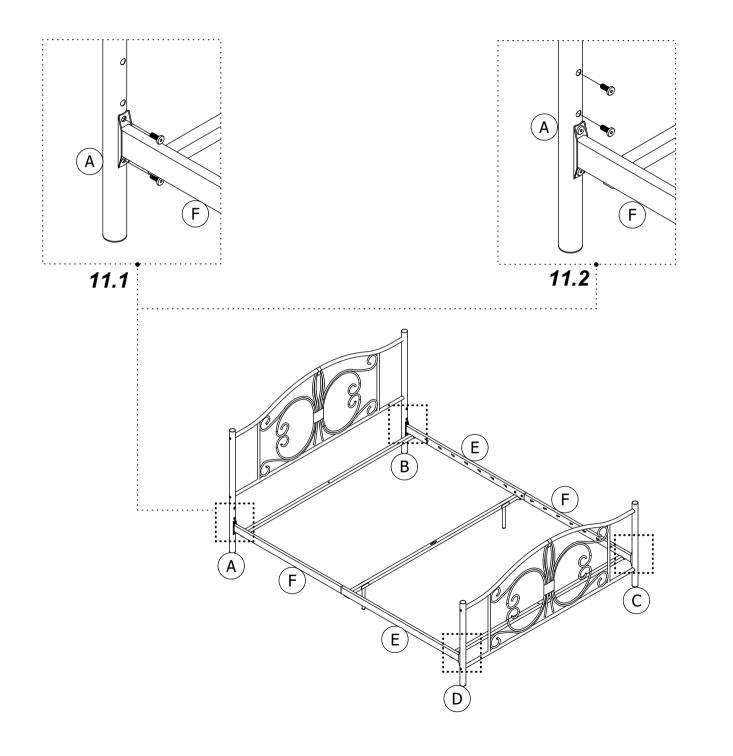
11.1 Attach sub-assembly E/F from previous step to A, B, C and D with 4.
