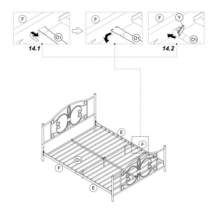
*14.1* Insert O1 into E X 2 and F X 2 as illustrated.*14.2* Lock O1 into place with Y.
