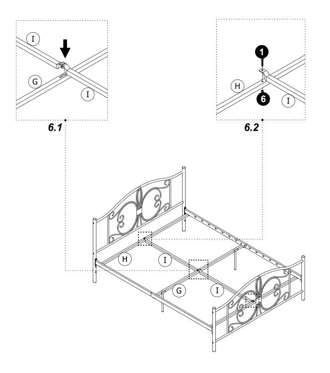
6.1 Insert one end of both I into the slot on G as illustrated.
