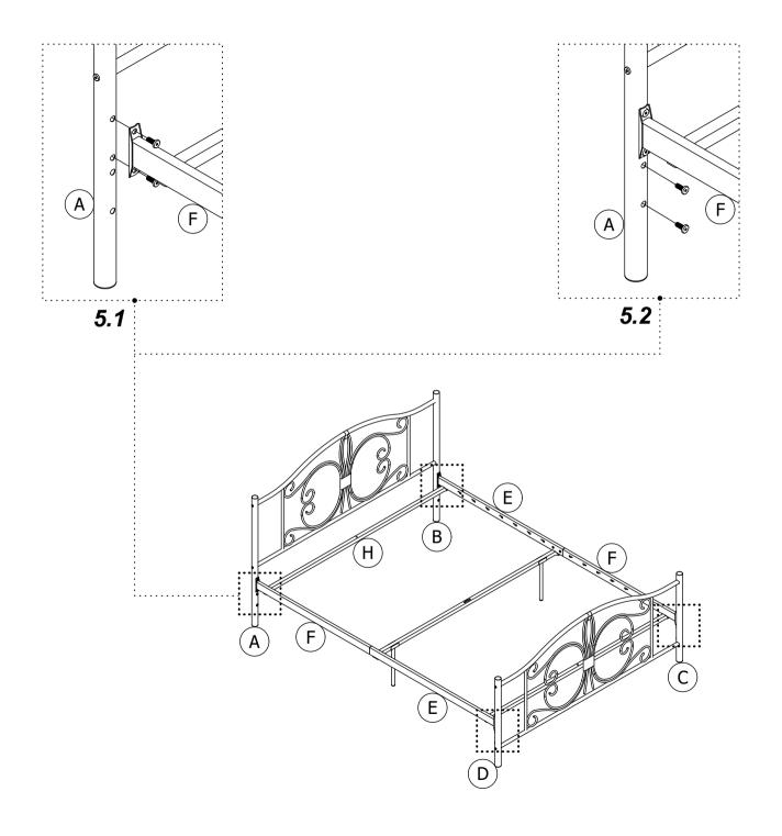
5.1 Attach sub-assembly E/F from previous step to A, B, C and D with 4.
