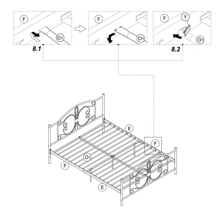
8.1 Insert O1 into E X 2 and F X 2 as illustrated.8.2 Lock O1 into place with Y.
