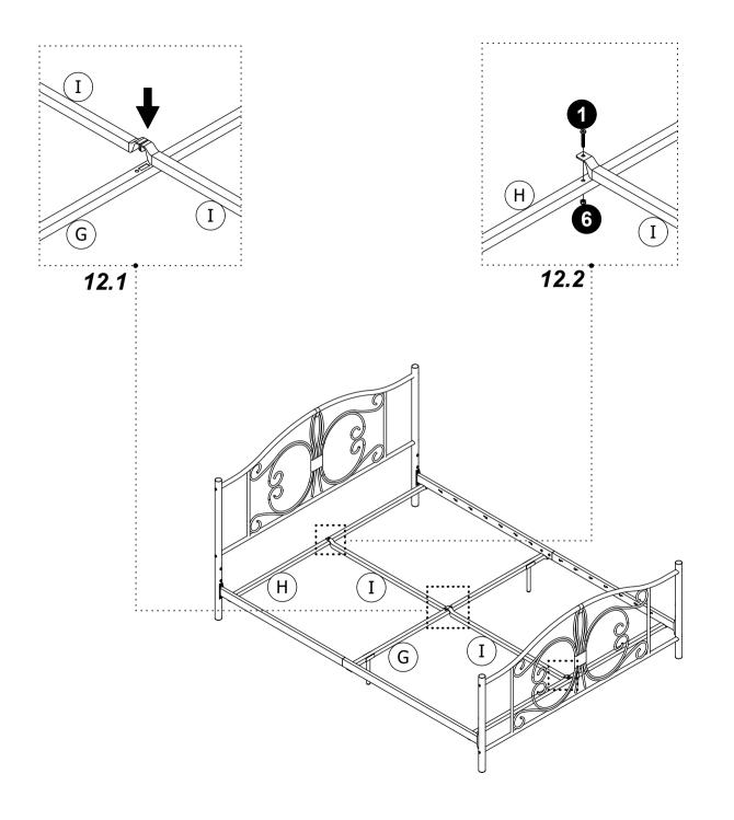
12.1 Insert one end of both I into the slot on G as illustrated.
