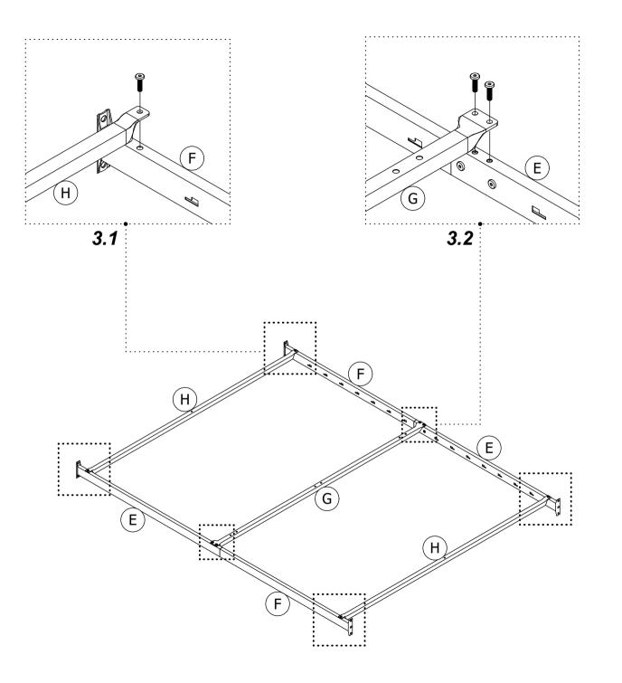
3.1 Attach H X 2 to sub-assembly E/F x 2 from previous step with 3.
