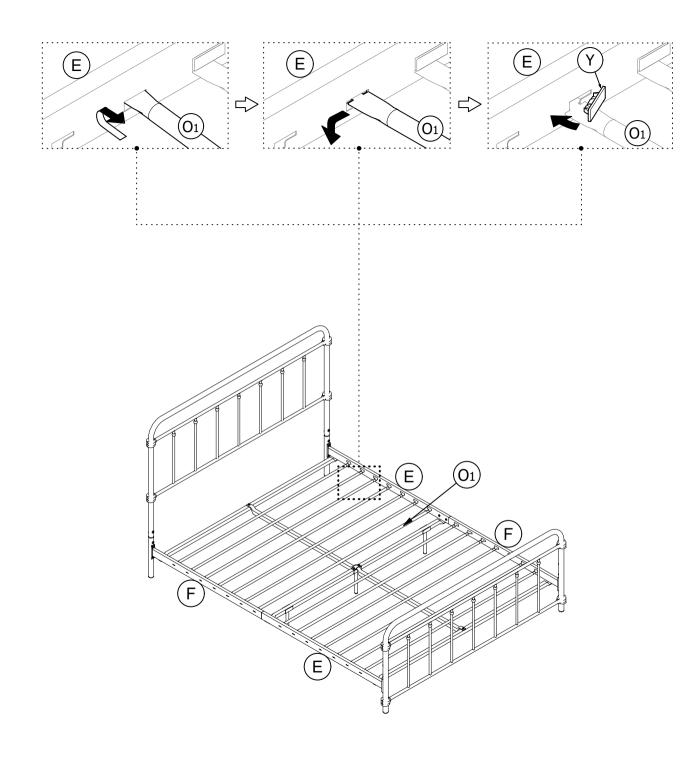
Insert O1 into E & F as illustrated, then lock O1 into place with Y.
