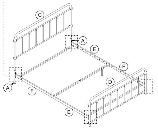
Attach sub-assembly **E/F** from previous step to **A** X 2 and **D** with **3**. Screw **3** into **A** X 2, **C** and **D**.
