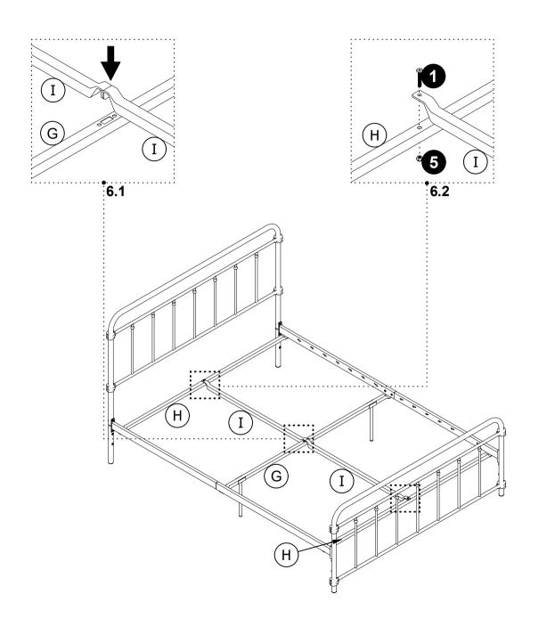
6.1 Insert one end of both I into the slot on G as illustrated.
