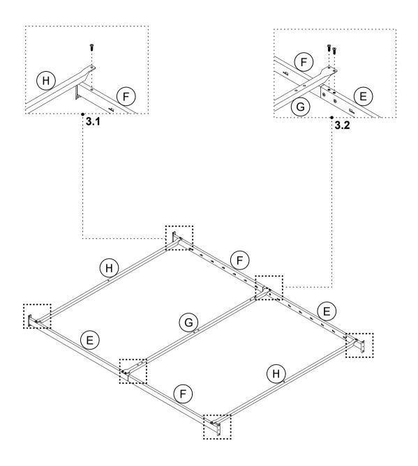
3.1 Attach H X 2 to sub-assembly E/F X 2 from previous step with 2.
