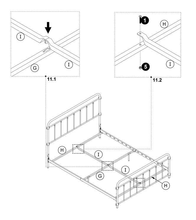
11.1 Insert one end of both I into the slot on G as illustrated.
