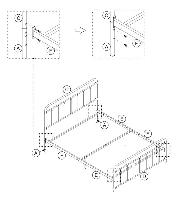
Attach sub-assembly **E/F** from previous step to **A** X 2, **C** and **D** with **3**. Screw **3** into **A** X 2 and **D**.
