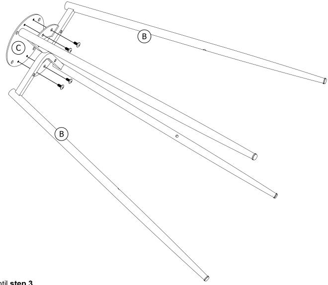
1. Do **NOT** fully tighten bolts at this step until **step 3**.
