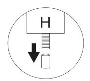
NOTE: remove the protective cap on support leg (H) before beginning assembly.
